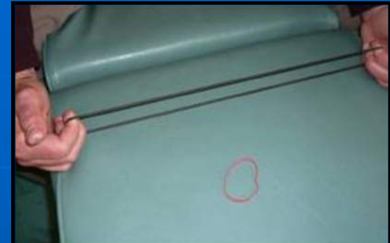
Excess tension, band will fatigue & become lax
